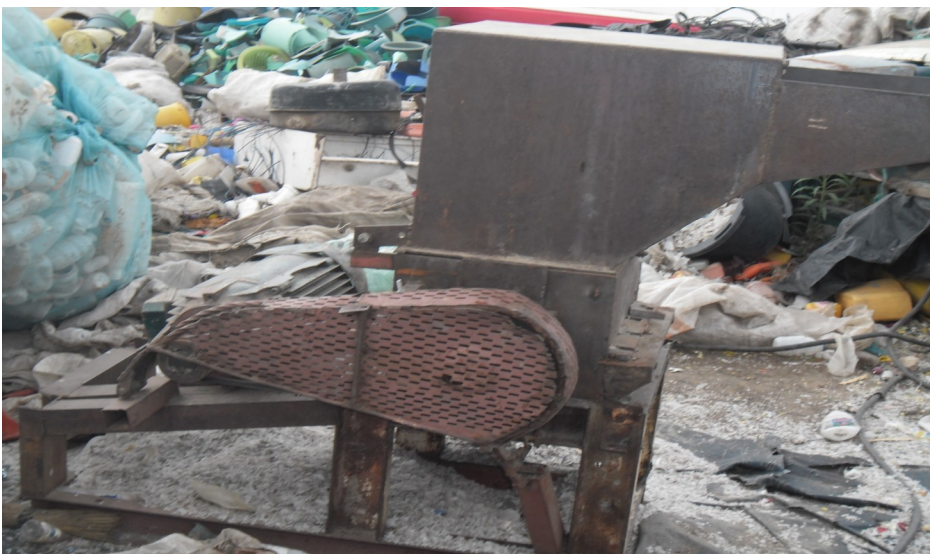
One of the home made chippers used by Innocent Chasvinura in plastic recycling
